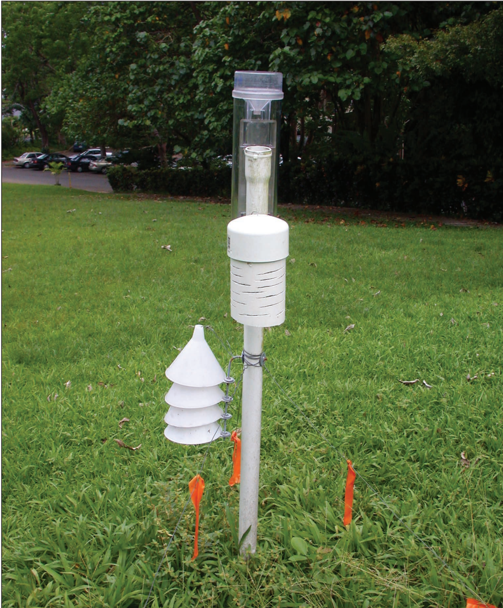
Figure 39—Climatological data sensors (temperature and rainfall) are part of a climate station operated by the Institute in front of the Institute building.
