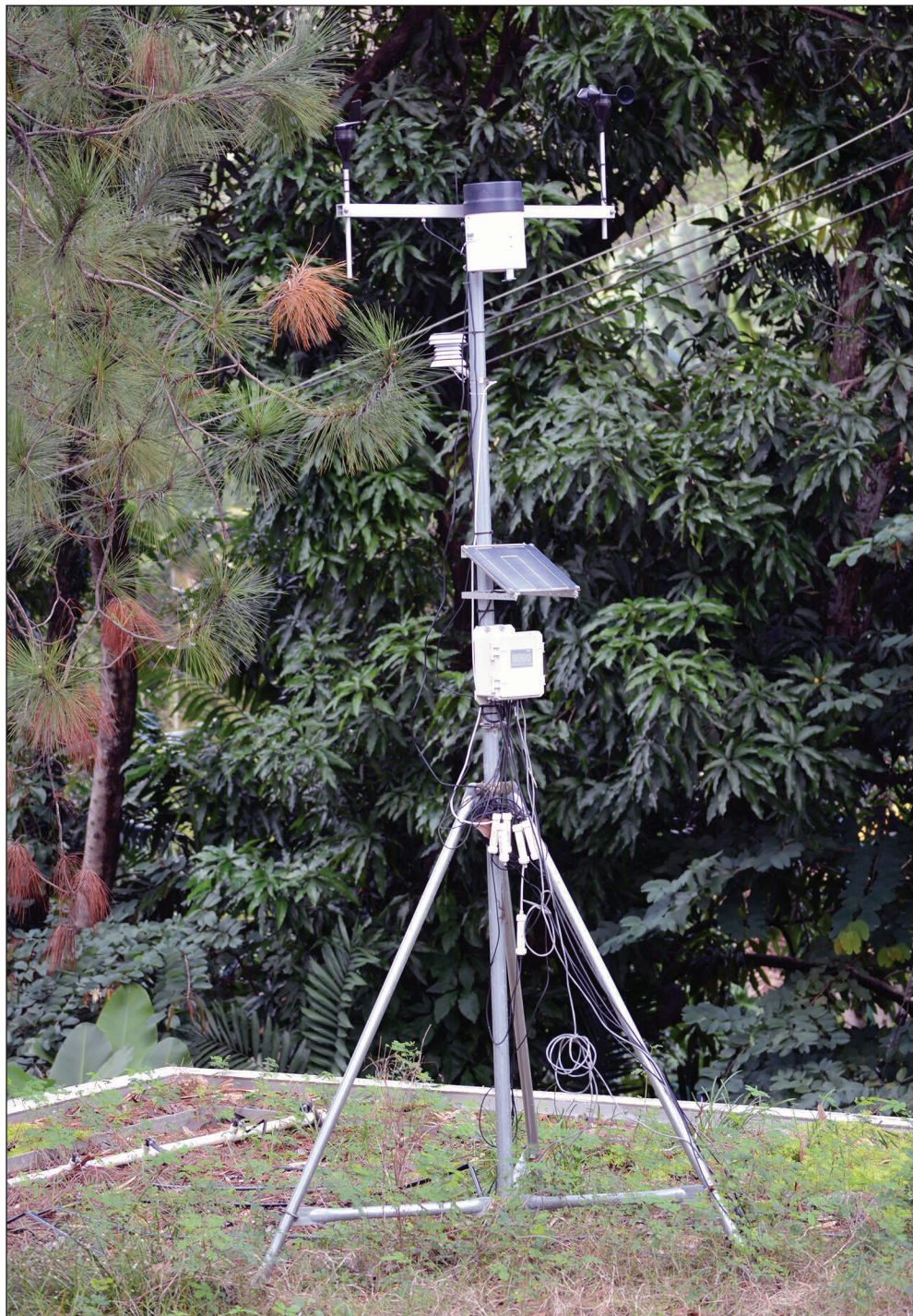
Figure 38—One of two Campbell weather stations on the green roofs. These stations monitor air temperature and humidity, wind speed, energy incidence, and rainfall.
