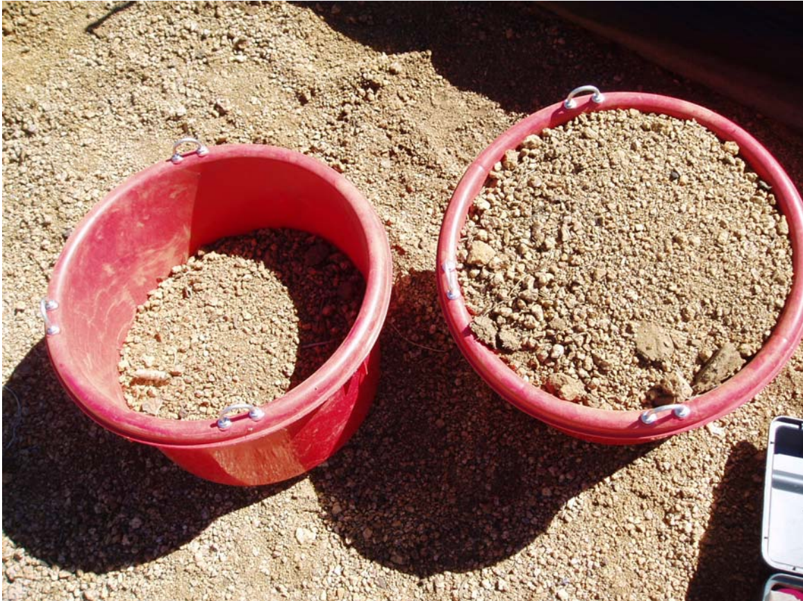
Figure 3. Graduated buckets used to measure excavated material from silt fence sites.
