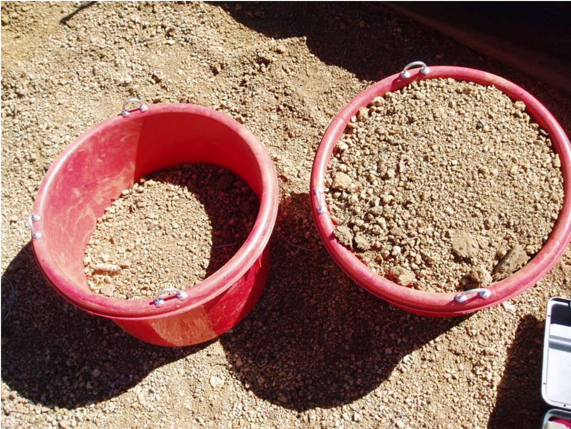
Figure 1. Graduated buckets used to measure excavated material from silt fence sites.
