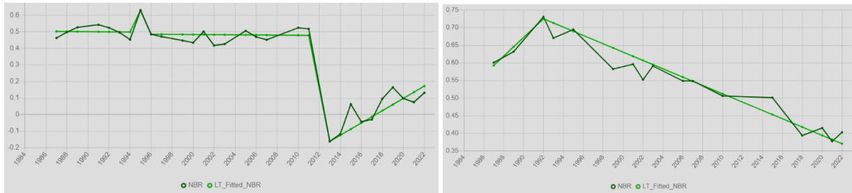
Figure 7. An example of raw medoid composite and LandTrendr fitted normalized burn ratio (NBR) values for a single pixel. The pixel depicted in the left chart shows a fire event, while the right chart shows insect-related tree mortality.
