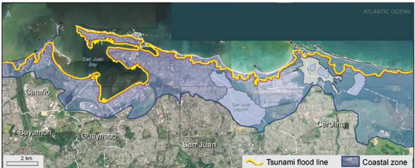
Figure 20. Trace of the expected inland penetration of a tsunami in the San Juan Metropolitan Area. The maximum runup wave level was estimated at 8.99 m. This information was provided by a Federal Emergency Management Agency/University of Puerto Rico Mayagüez Campus study sponsored through Sea Grant.
