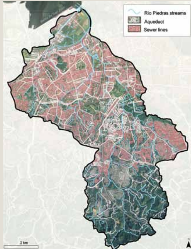
Figure B2-4. Network of pipes (potable water in white and sewer lines in red; stormwater not shown) in the Río Piedras River Watershed. The watershed is delineated with a black line; the surface river channels are in blue. Data are for 2006. The infrastructure is managed by the Puerto Rico Authority of Sewers and Aqueducts. The Geographic Information System layer data set was obtained from the Puerto Rico Highway Authority.
