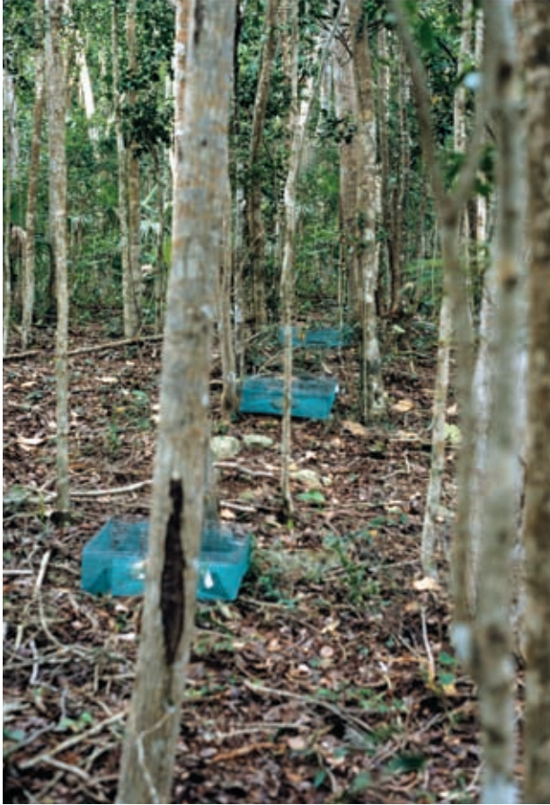
Litterfall baskets used during the productivity study in dry evergreen woodland on ridge plot #13, Cinnamon Bay watershed (February 1992).
