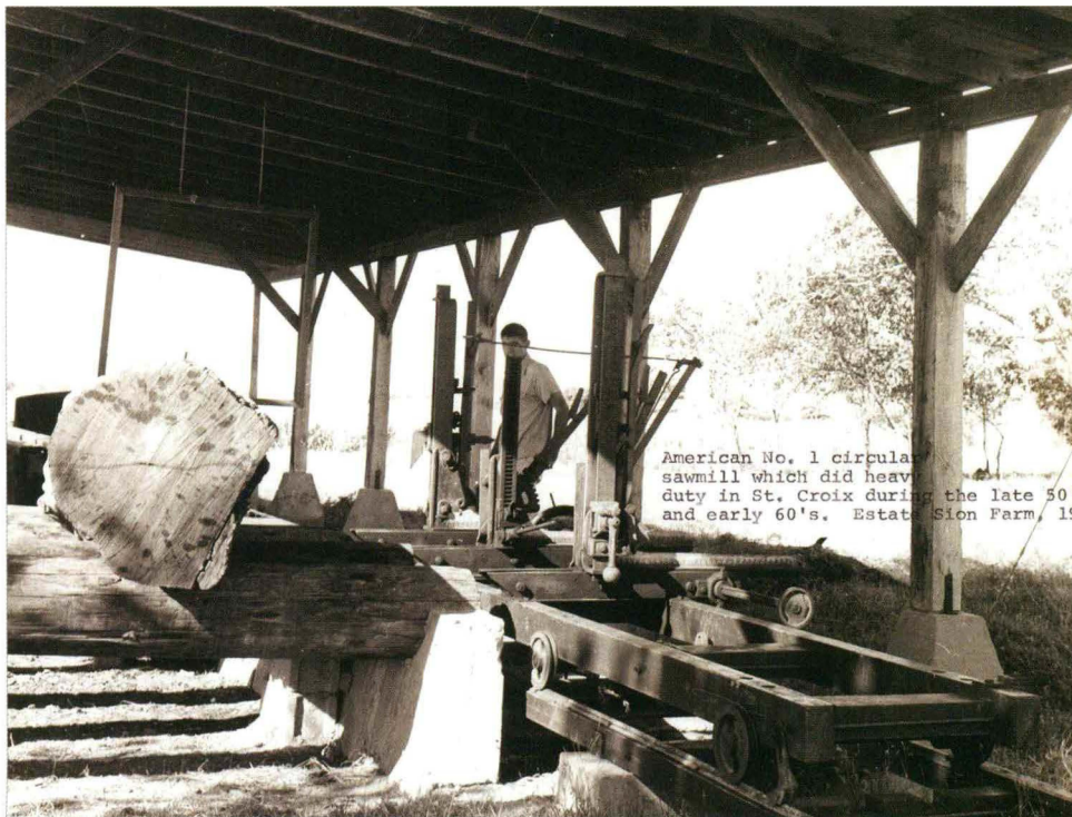
American No. 1 circular sawmill operated by the U.S. Department of Agriculture Forest Service on Sion Farm during the late 1950s and the early 1960s.
