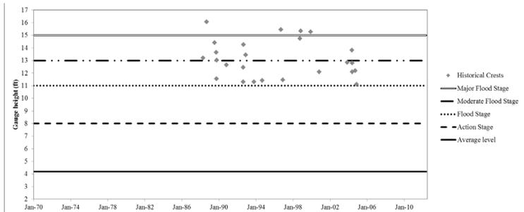
*Figure 2: Historical flooding events registered at the USGS gauging station located at El Señorial (Station No. 50048778) in the higher part of the watershed*
