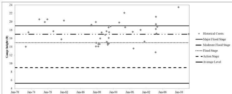
*Figure 3: Historical flooding events registered at the USGS gauging station located at Hato Rey (Station No. 50049000) in the lower part of the watershed*
