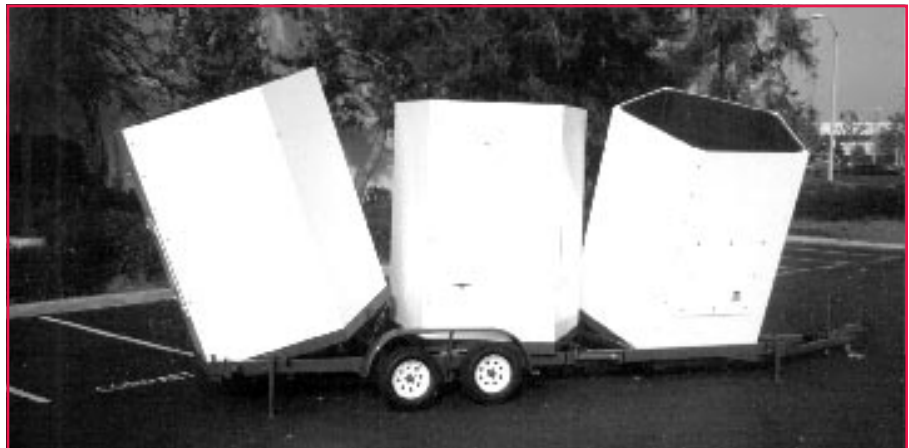
Figure 1. —The 8-foot- (2.4-m-) tall, foam- and lead-lined wooden enclosures that surround SODAR's antennas and drivers mounted on the trailer that transports them to the field. The enclosures dampen SODAR's sound pulses and reduce the impact of background noises to increase the sensitivity of its measurements. Photo: Ken Underwood, AeroVironment Inc., Monrovia, CA, 1996.
