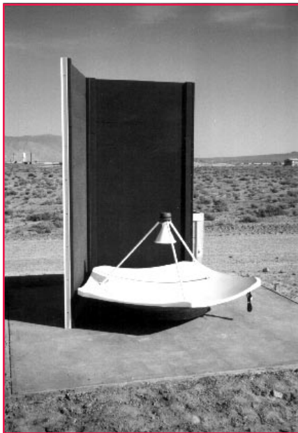
Each SODAR antenna consists of a parabolic dish that faces upward with an acoustic driver mounted above each dish pointing downward. By emitting a sound pulse at a known frequency and monitoring the Doppler shift of the return echoes, the instrument calculates the windspeed and wind direction at various altitudes. Photo: Jeff Bradley, AeroVironment Inc., Monrovia, CA, 1996.
